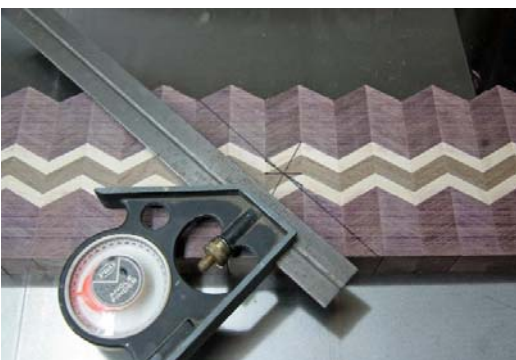
16. Use a combination square to draw a line showing where the next cut is to be made.
