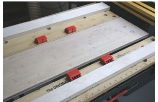
12. A Workmate 425 can form a channel that will align the strips.
