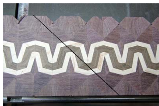
25. Use a combination square at 45° to mark the intended path of the next saw cut.
