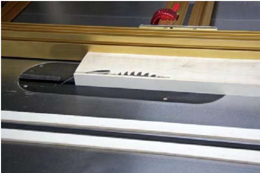
6. The INCRA TS-LS Table Saw Fence is the safest and most accurate way of cutting thin strips.
