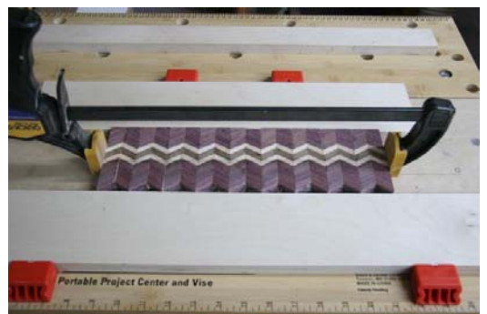
13. Tighten the clamps, alternating between the channel clamp and the end clamp.
