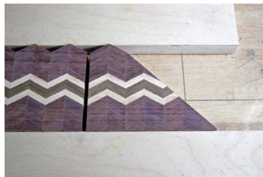
23. Glue the remainder of the board just cut to the front of the next board to be cut to eliminate waste.
