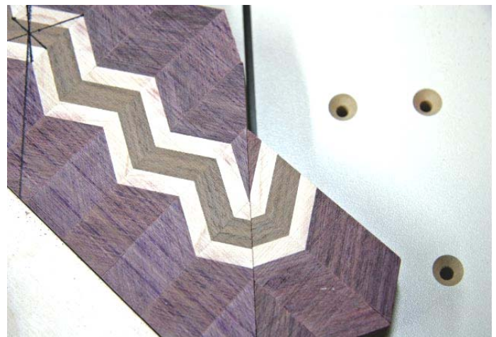
20. Use the cutoff to check the pattern it makes. If the pattern is not symmetric, make minor changes to the registration point.
