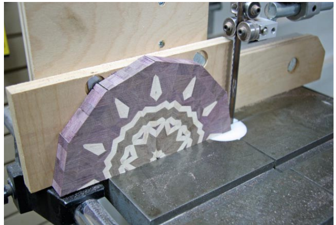
30. Make test cuts on scrap wood to make sure that the blade position is correct and that the blade does not wander.
