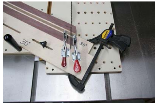
11. A dedicated 30° fence is aligned with a commercial angle guide (in yellow).
