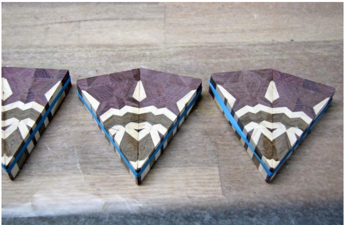
29. The radial segments are first glued into pairs and then the pairs are glued together to make the half-discs.
