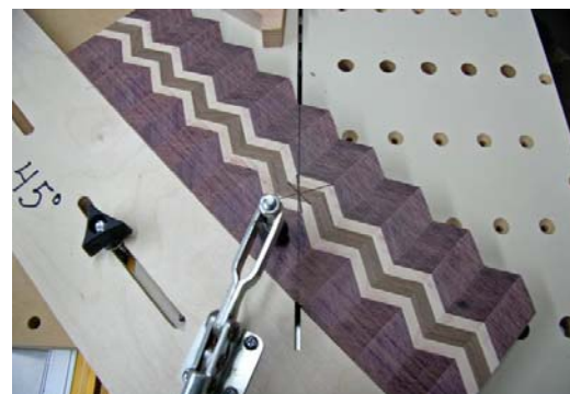
17. The board has been positioned so that the line is centered in the saw kerf of the sled.
